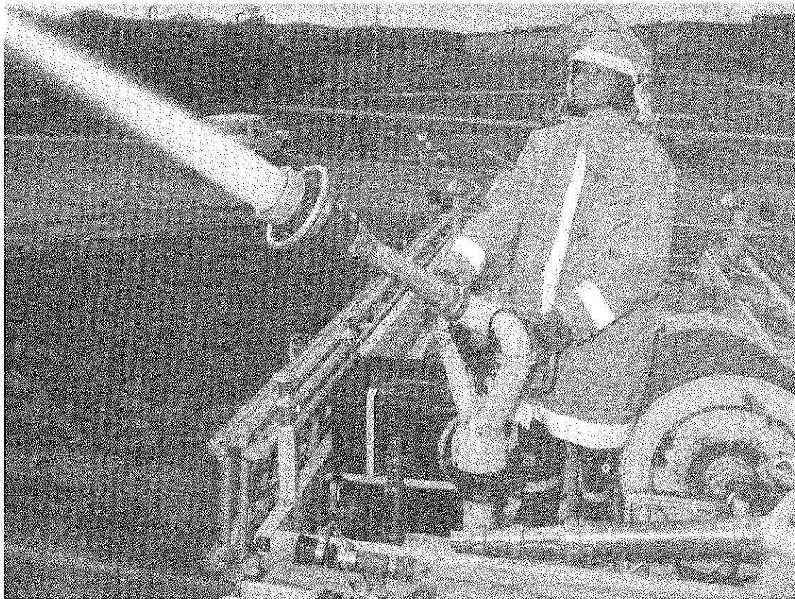
Debra D. Hannah, Clerk IV (D-334) gained hands-on experience in firefighting techniques by operating the Portsmouth Fire Department's deluge gun, which is capable of delivering 1,250 gallons of water per minute.
